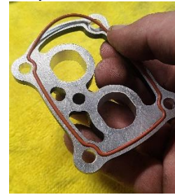
Picture 2. O-ring installs in cut groove on bottom of anti-rotation plate.
